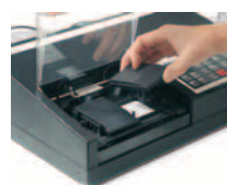
Fig 9. Simple blotting procedure of PhastTransfer.
